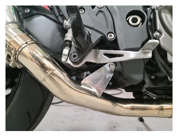
Mount your new Lextek Silencer to the header and line with the mounting point on the pillion peg. Using the OEM bolts secure the silencer, use a spacer (supplied) if needed.
