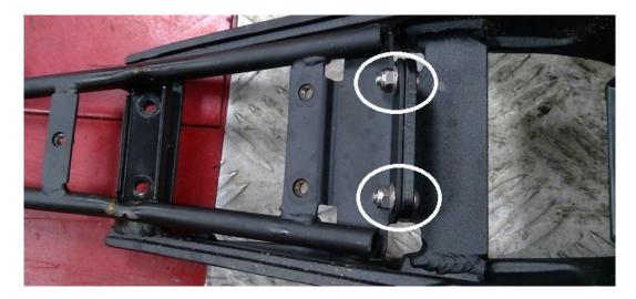
10. Once removed, cut the subframe just behind the rear mounting bracket as shown.
