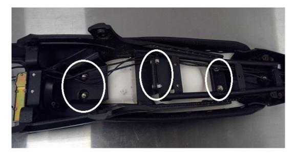
12. Assembly the tail tidy assembly including indicators and original rear light unit. It is recommended to fit the indicator brackets to the "front" of the tail tidy unit using the bolts provided to prevent interference when mounting the number plate.
