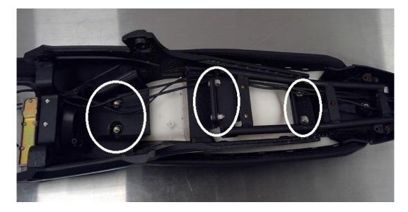
7. To separate the rear panel from the subframe, first remove the 2 screws securing the pieces together.
