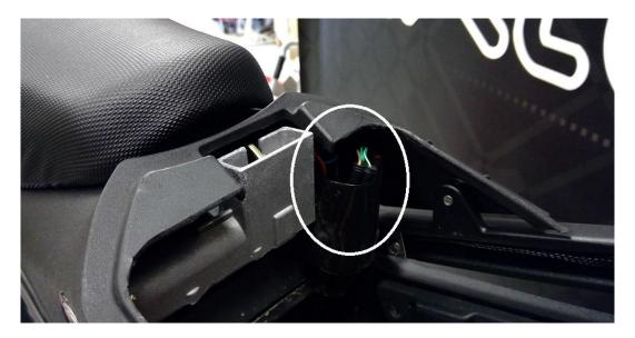
4. Remove the 2 bolts (M6  $\times$  10mm) from the fairing panel followed by the 4 bolts (M8  $\times$  20mm) securing the assembly to the chassis.
